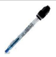
The ALS-PHTA1 sensor is a top of the line autoclavable, steam sterilizable pH and temperature sensor. Ideal for Sterilize In Place (SIP) and Clean In Place (CIP) applications. It withstands temperature of up to 140 deg C and pressure up to 6 bar. Pressurized electrolyte extends the life of the sensor. Available in lengths from 120 mm to 425 mm.
